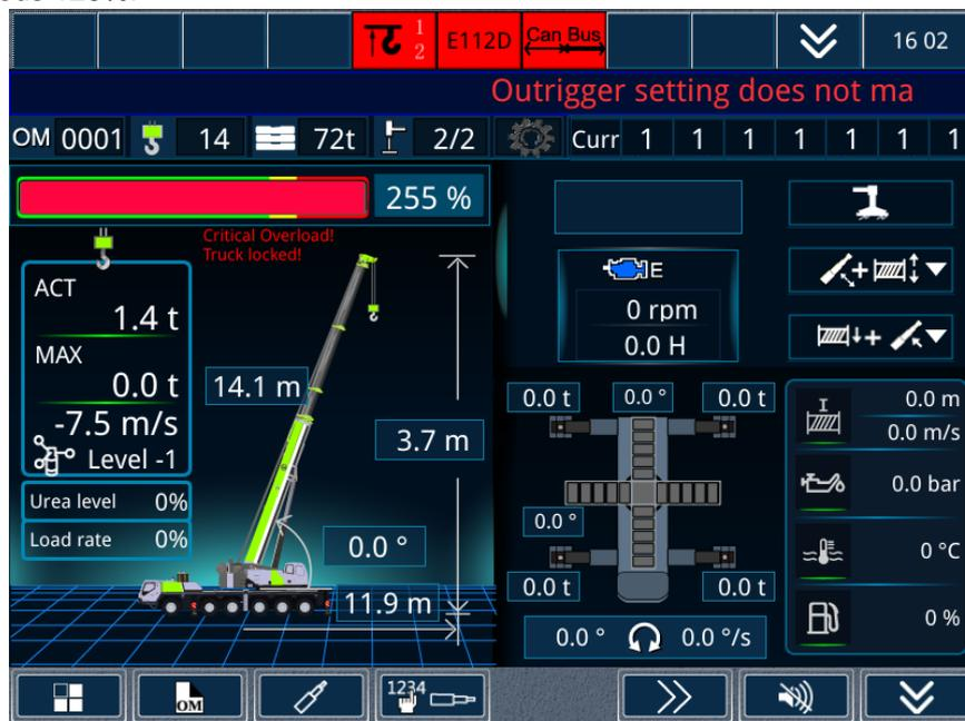
Figure 4-44 Main interface serious overload warning prompt
