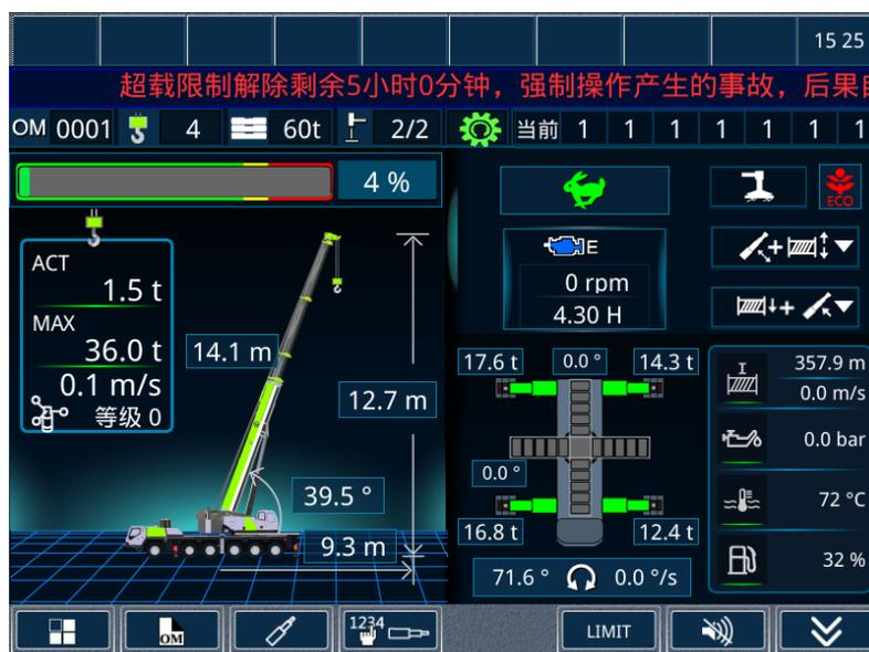
Figure 4-47 Remaining unlocking time display, main interface
