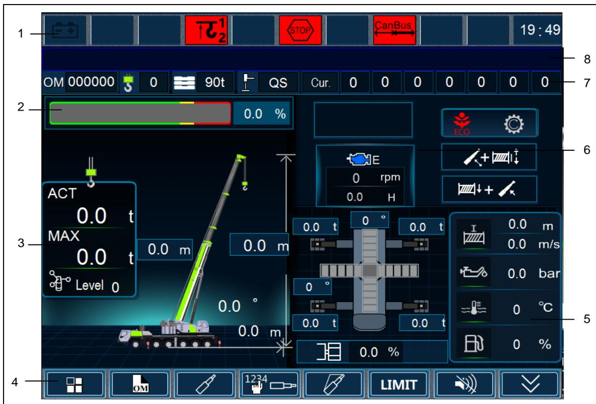
Figure 4-11 Crane working status monitoring interface
