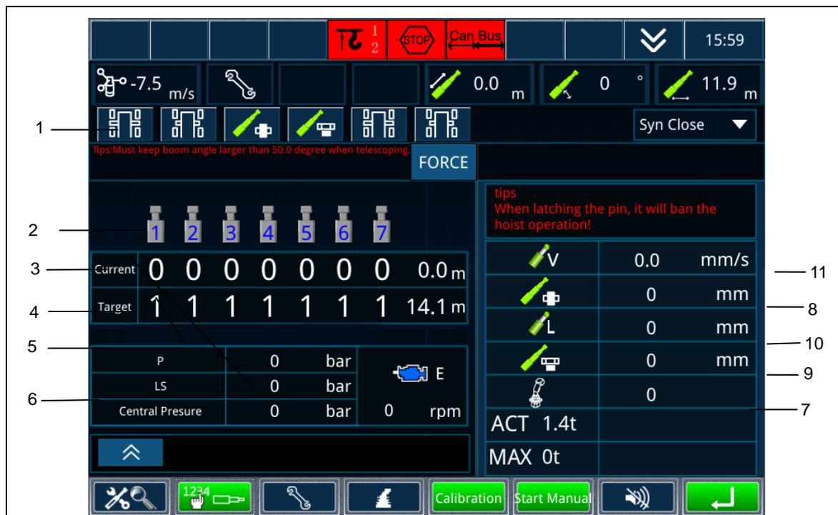
Figure 4-38 Boom status during manual telescoping
